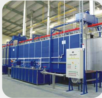
7-Tank Pretreatment Process
